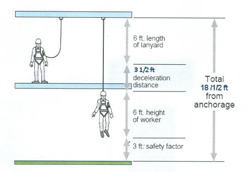
How to determine total fall distance with a shock-absorbing lanyard.
